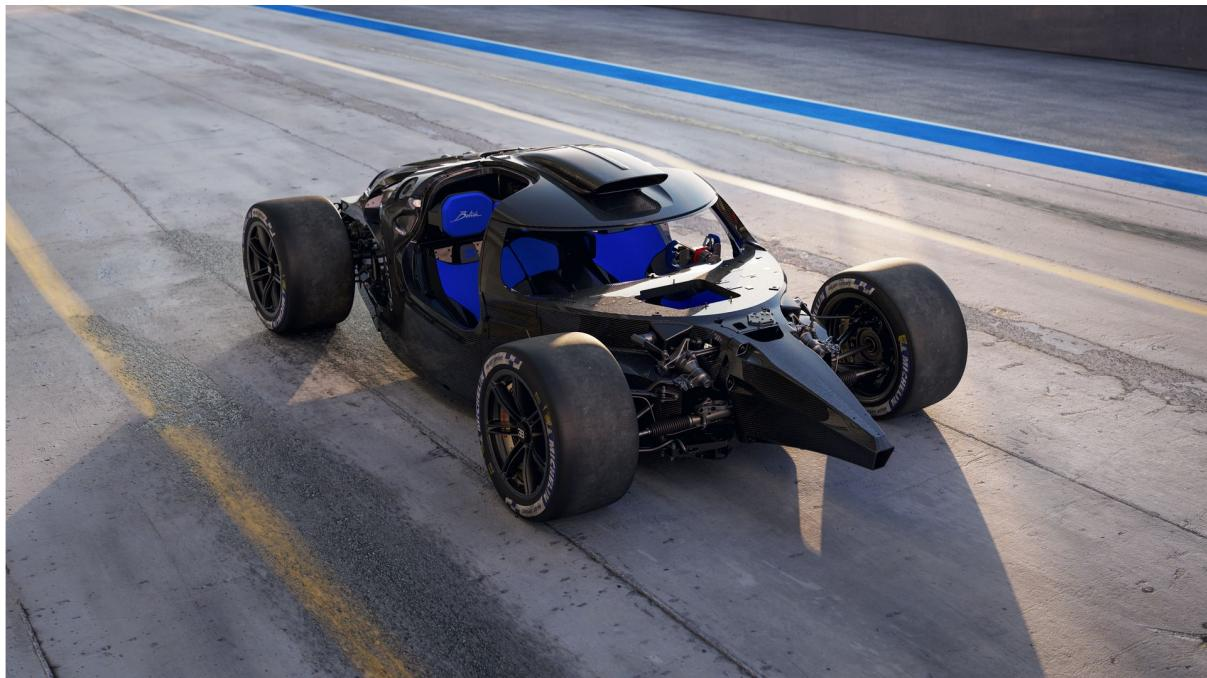
Along with incredible power, precision and performance, a track-only hyper sports car must possess exceptional levels of safety, which is why the Bugatti Bolide features an innovative new carbon fiber monocoque developed to the same demanding Fédération Internationale de l'Automobile LMH and LMDh requirements as Le Mans race cars.
