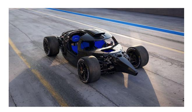
Along with incredible power, precision and performance, a track-only hyper sports car must possess exceptional levels of safety, which is why the Bugatti Bolide features an innovative new carbon fiber monocoque developed to the same demanding Fédération Internationale de l'Automobile LMH and LMDh requirements as Le Mans race cars.
